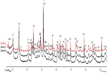
Fig. 2. Diffractograms of the mine wastes from the coal mine "Bogdanka" Description: Ch - chlorite, I - illite, K - kaolinite, Ka - calcite, P - pyrite, S - siderite, Sk - feldspars, Q - quartz
