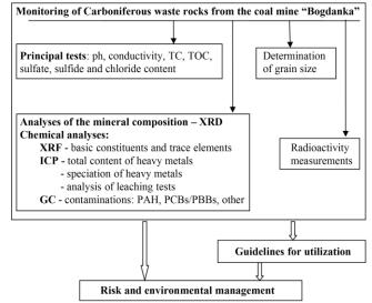
Fig. 1. Diagram of the monitoring system of the carboniferous waste rocks from the "Bogdanka" coal mine
